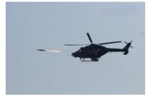
Imaging Infra-Red Seeker, has been established, which will enable the induction of the 'Helina' into the Armed Forces. 'Helina' is the third generation, fire and forget Anti-Tank Guided Missile that can engage targets both in direct hit mode as well as top attack mode. The system has all-weather day and night capability and can defeat battle tanks with conventional armour as well as with explosive reactive armour.
